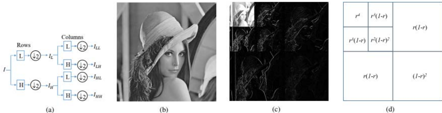
Fig. 2. The process of the DWT and the transformed example: (a) The process of the DWT, where downward arrows mean down-sampling. (b) The original image. (c) The result of the two-times DWT. (d) The ratios for different patches.
