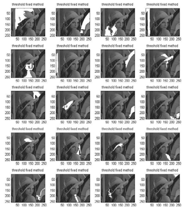
Fig. 11: The result of segmentation with adaptive threshold in (16) for Lena image
